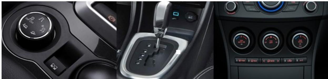
Automotive manufacturers may source the various cockpit sub-assemblies from different suppliers. It is very important to have tight tolerances as well as standardised test set-ups to ensure correct colour matching and homogeneous intensity outputs of each sub-assembly. This ensures the consumer does not perceive colour and intensity non-uniformity in the end product.
