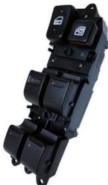
Automotive manufacturers are extensively using LED backlit switches and panels to create a safe and aesthetically pleasing cockpit environment for a car's occupants. Steering wheels are being designed with safety in mind to include more of the controls for in-car entertainment, phones and cruise control. Panels and switches with etched or painted symbols backlit with LEDs are nearly invisible during the day but give the driver better orientation and sense of space while driving at night.
