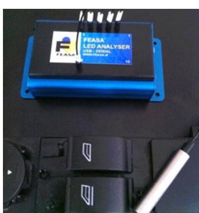
Feasa's Low Light Led Analyser is the ideal solution for these applications. The extra sensitivity measures low light levels after the light has passed through an etched plastic panel.
